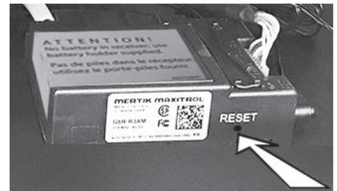
3. Within the subsequent 20 seconds, press the small flame button (🔥) on the remote handset until you hear two short beeps confirming the synchronization is set. If you hear one long beep, this indicates the code learning sequence has failed or the wiring is incorrect.
