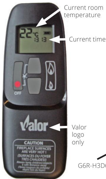
The non-thermostatic (NT) handset is identified with a Valor logo only. It shows the current time and room temperature. The number shown on its back cover label is G6R-H3D6
