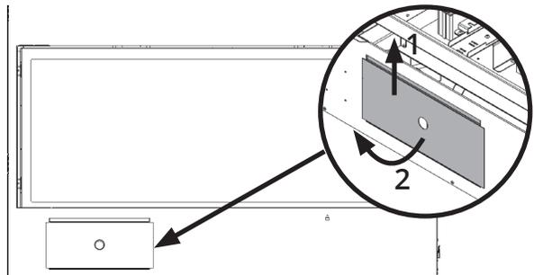
1. Locate and remove the bypass screw from the valve and discard (this screw may be covered by a sticker). Note the bypass screw may require either a flat head screwdriver or an Allen key depending on its type. After unscrewing it, the bypass screw may need to be pulled out using pliers as there is an O-ring retaining it within the valve body.
