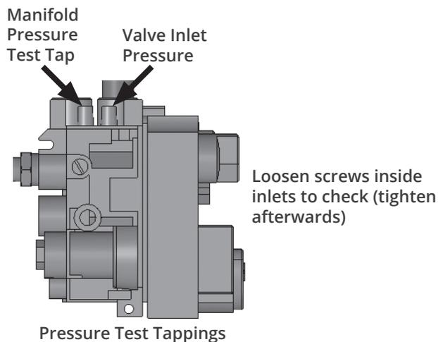
2. Light the appliance and turn the control to full input.
