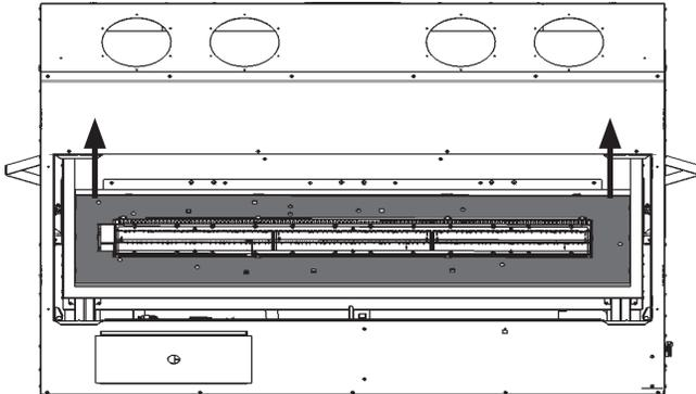
5. Remove the burner by undoing 5 screws, then slide the burner to the right to disengage it and lift it out.
