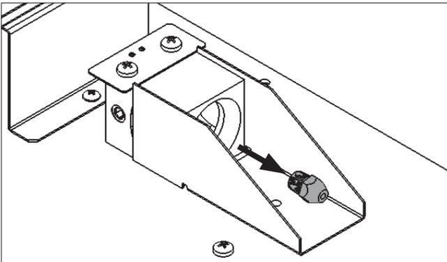
2. Replace the old injector with the new injector from the kit using the socket wrench to tighten. Use thread sealant when installing the new injector.
