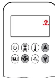
**NOTE:** SETTING only. Fan is switched on automatically when gas opens. Circulating fan has 4 speed levels from low (1 bar) to high (4 bars).
