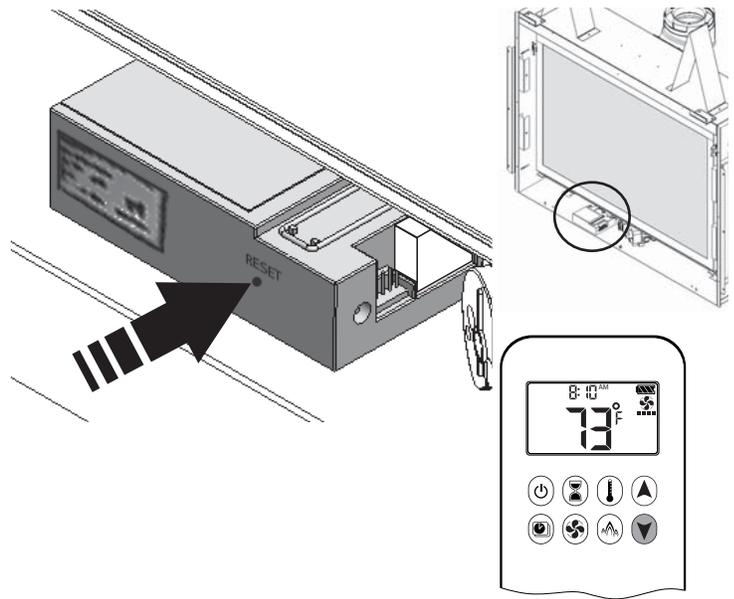
**NOTE:** Before using the remote control system for the first time, the receiver and the handset must be paired. See the section *Remote Control Initial Pairing* on page 61 of this manual.
