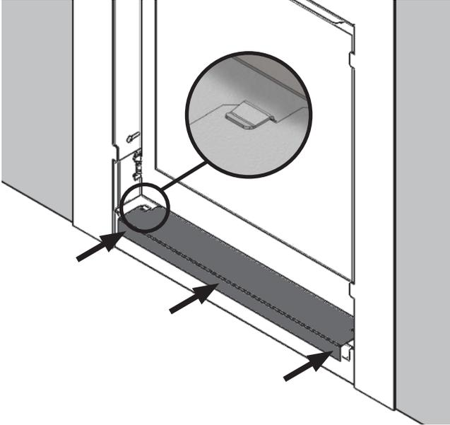
2. Hang the front assembly on the four tabs in the backing plate assembly.
