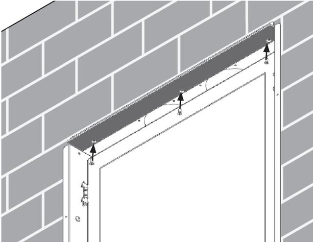
2. Locate the backing plate assembly inside the perimeter of the appliance's opening and press it firmly against the wall finish, as far as it will travel. Secure the plate using 4 black low profile screws (included).
