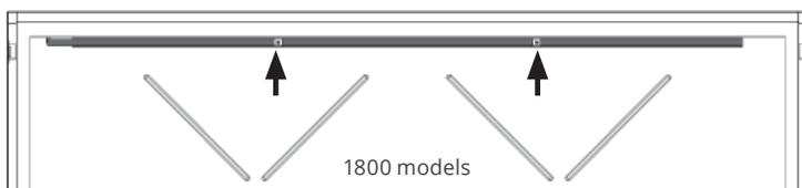
5. Place the rear glass retainer strips, groove at the back, on the ledge of the firebox behind the burner. The strip are held in place with the tabs of the ledge as indicated below.
