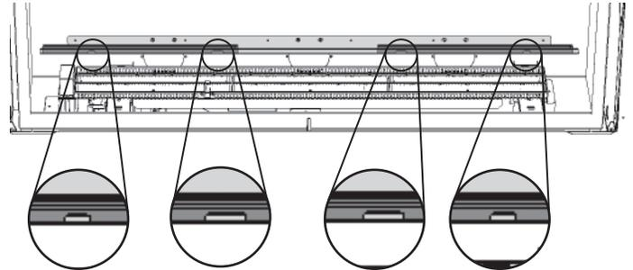
6. Insert, from the center of the firebox, the first rear panel section - left or right - behind the top rail and place in the groove of the retainer strip. The left section will overhang the strip on the left. The right section will overhang the strip on the right. The center section straddle both strips.
