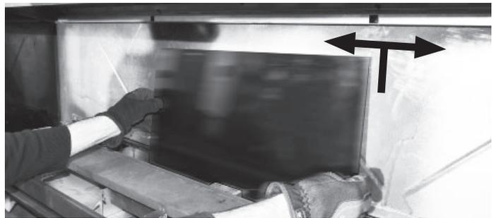
7. Insert the second section in the groove of the retainer strips and slide it to the opposite side.
