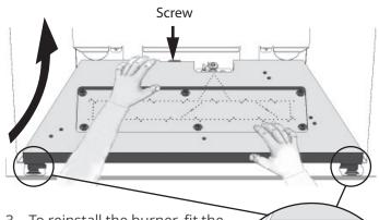
3. To reinstall the burner, fit the burner in the firebox inserting the front tabs first in the lances.
