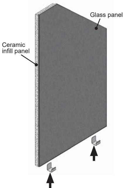
3. Place the rear ceramic filler panel on the railing at the back of the firebox and add the glass panel, smooth side out, in front of the ceramic panel. Both panels should be retained at the bottom by the flange of the railing. Hold the panels in place.
