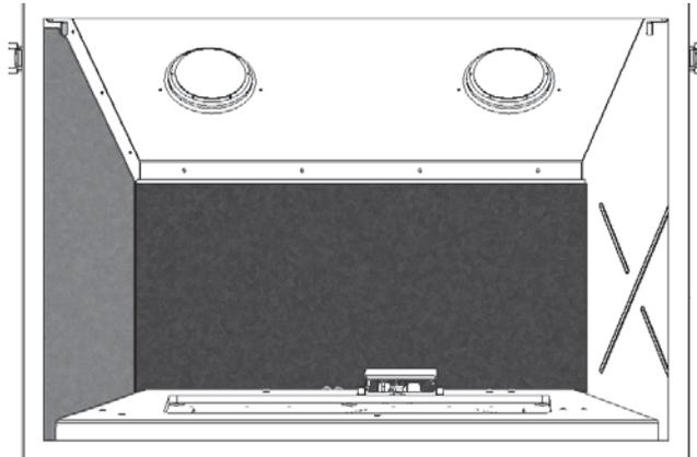
5. Rotate the side anchor over the top edge to hold the panels ensuring the panels are tight together. Tighten the anchor screw.
