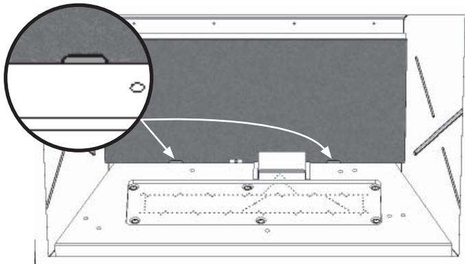
4. Install either the left or the right side glass and filler panels assembly against the firebox side and slide it back against the rear panels.
