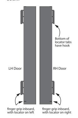
6. Position LH door to left side of front panel, identify door slots top and bottom just behind backing plate front face and slide door locator in position.
