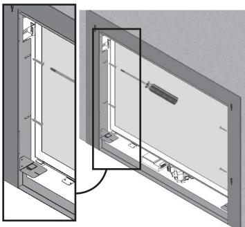
3. Slide the removable panel in the clip on the horizontal supports on each side and push it in until flush with the front trim.
