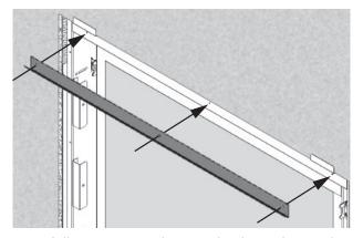
2. Carefully position and secure backing plate with 4 low profile screws to 4 firebox mounting brackets; before tightening, hold plate up against wall finish then tighten.
