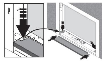
4. Adjust the position of the convection brackets on each side of the window. Release the nut, pull the bracket as forward as possible and tighten the nut.
