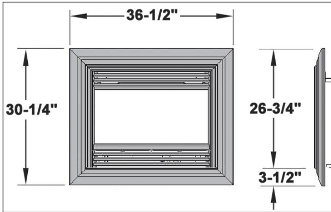
The Contour 4-Sided Trims 748CTK (black) and 749DTK Deluxe (black) are intended to be used on any Valor G3 738 or 739 appliances, or on a Retrofire RF24B when installed in a RA24ZC Zero Clearance Kit fitted with any inner front.
