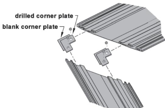
2. Attach the 2 trim mounting brackets to the side trim pieces with 3 screws for each side. The brackets should be flush to the bottom inside corner as indicated.
