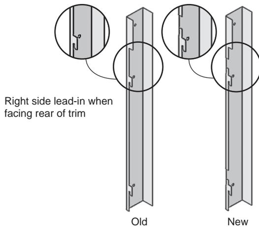
4. Install the new side lead-ins provided with the barrier screen (3 nuts per side) (709 only).
