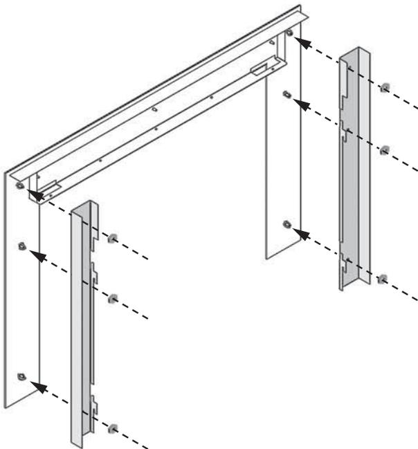
5. Hook the barrier screen to the back of the front. Orient the screen so its tabs are on the back.
