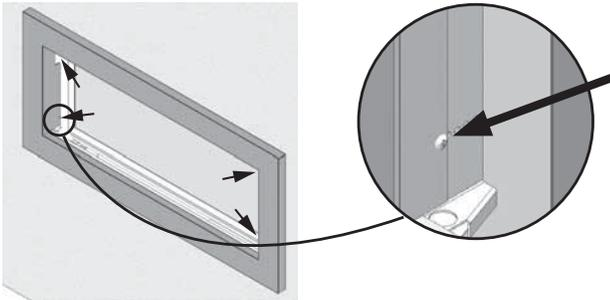
3. On the back of the trim, remove the top bracket (4 nuts).
