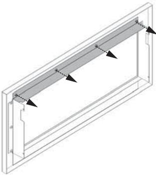
4. Install the new top bracket to the back of the trim provided with the screen (4 nuts).
