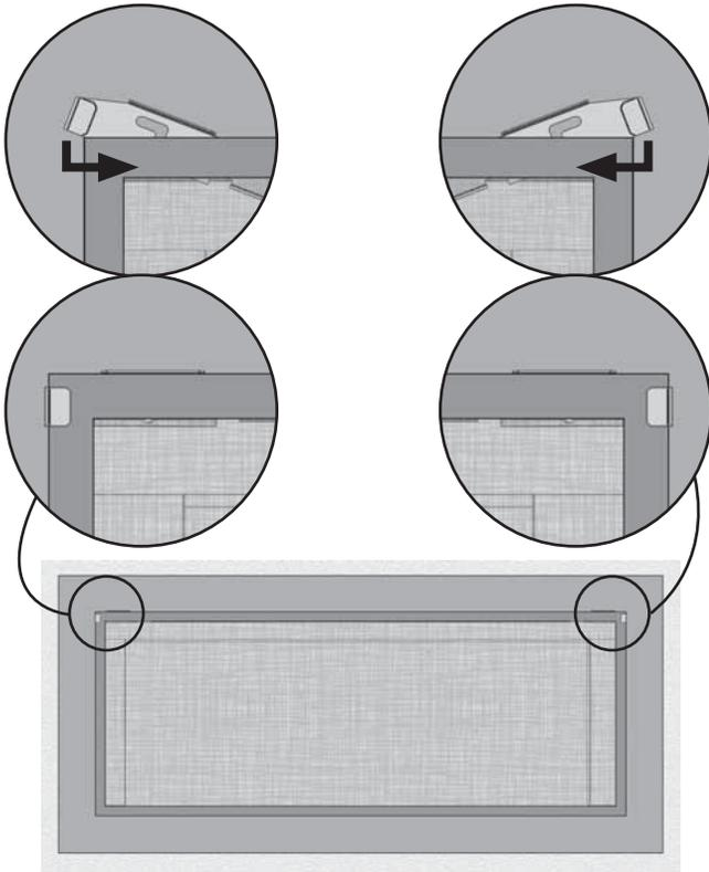
**Note:** The levers hook in the slots of the new top bracket installed earlier as show below.
