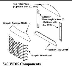
Model 540 WDK is required for all 922 Adorn Fireplace installations fitted with 539/549 Windsor Arch Cast fronts.
