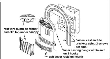
**Step 4** – Fasten casting to brackets on firebox and hang inner casting within arch on 2 hooks. Install wire guard as shown.
