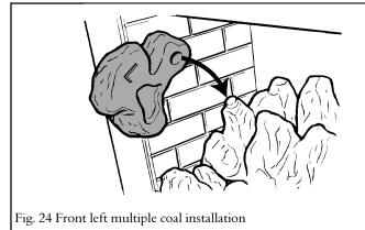
the block must locate in the round peg at left of the base coal (See figure 24).
