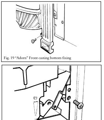
Fig. 20 "Visage" Front surround bottom fixing
