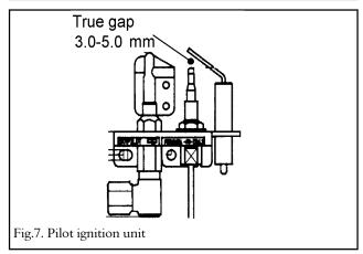
Sparks should be seen tracking from the electrode pin to the thermocouple tip (see figure 7).
