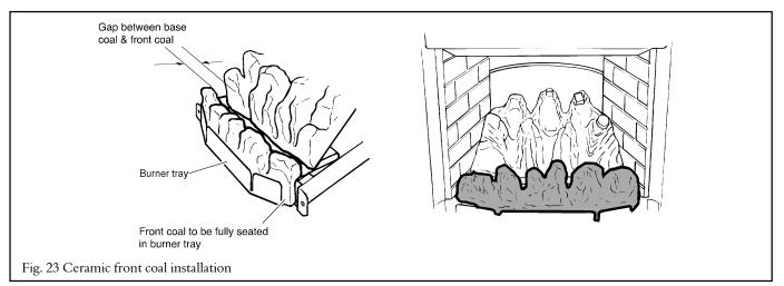
13.3 Find the front left multiple coal block. It is marked "L" underneath. Place it at the left side. The hole in
