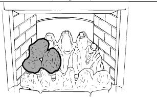
**13.4** Find the front right multiple coal block. It is marked "R" underneath. Place it at the right side.
