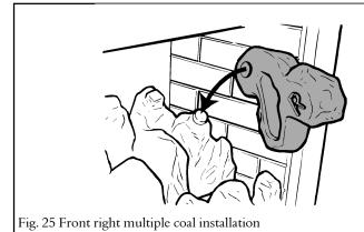
**13.5** Find the rear multiple coal. It has a square hole underneath. Place it centrally behind the front
