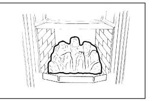
There will be a gap between the rear of the front coal and the front of the base coal (See figure 23).
