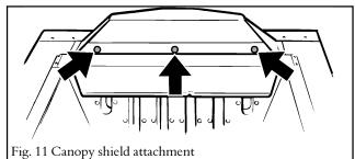
7.6 <u>"Visage" front only</u> Fit the two surround securing brackets to the convection box side flanges with the screws supplied. Be aware of the different orientation of
