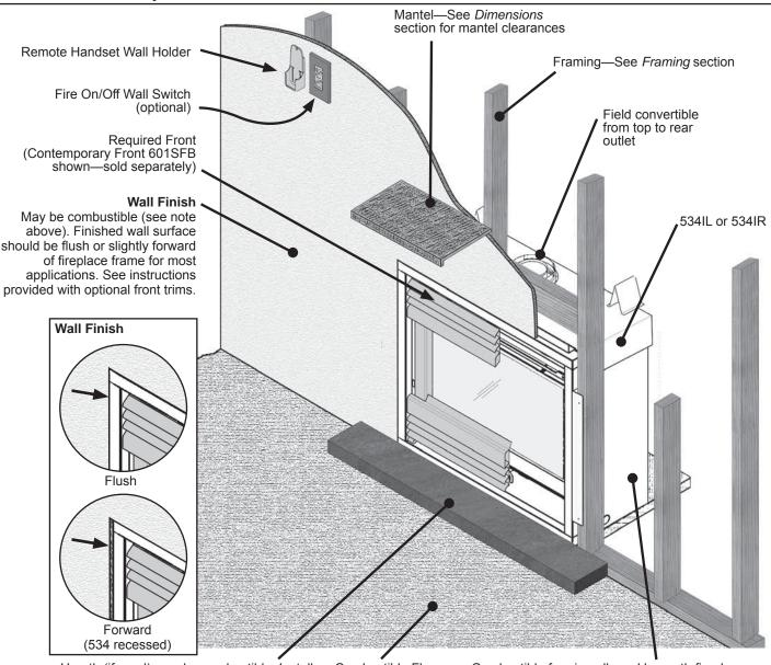
Hearth (if used) may be combustible. Install the bottom of the heater flush with the top of finished hearth for most applications. See instructions provided with optional front trims. Combustible Floor
