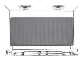
Hold the left hand side panel at an angle and insert its bottom edge inside the firebox. Rotate the panel to a vertical position ensuring that the top edge is behind the flange of the firebox. Pull the panel as forward as possible against the left edge of the firebox.
