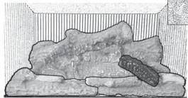
Identify the middle cross log. It does not have a hole underneath. Place its narrow end on the flat depression in the rear log next to the right cross log on the rear log. Place its wider end on the front log.
