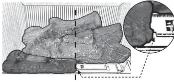
Place the front right log on the top of the burner with its left end abutted to the front left log and its front edge resting slightly on the window frame.
