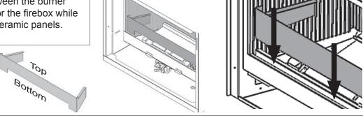
Place the rock ceramic base on the log support behind the burner. The front bottom of the base must rest against the vertical tab of the spacer brackets.
