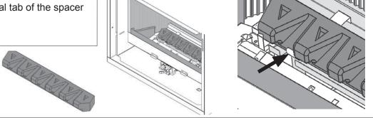
Install the ceramic platform in the firebox rotating down to insert the front first behind the Front Support. Lay the back of the ceramic platform against the rear ceramic panel again being careful not to scrape the ceramic panels.
