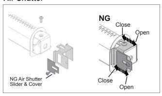
In a few unusual installations, the flame picture may be improved by adjusting the aeration. The need for adjustment should be determined only by operating the appliance with the ceramic rocks and window installed.
