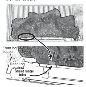
2. Place the front left log on top of the burner with its front edge resting slightly on the window frame.
