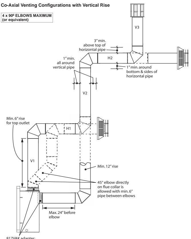
817VAK adapter: required for top outlet; required for rear outlet **except** when connecting the 551DVK terminal directly to the appliance.
