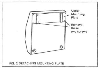
2. Mark the wall at the centers for the upper mounting holes. For accurate marking, place the upper mounting plate against the wall with its raised channels touching the wall and the holes in the channels towards the top. The bottom edge should be parallel with the floor. The minimum height from the floor to the bottom edge of the mounting plate must be 19½". With the plate firmly held against the wall, mark through the holes in the two raised channels onto the wall (fig. 3).
