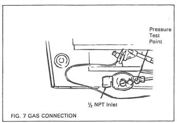
Check all gas piping and connections for leaks after installation or servicing.
